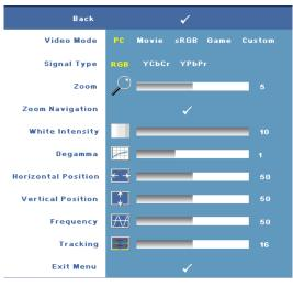
VIDEO MODE—Select a mode to optimize the display on how the projector is being used: PC, Movie, sRGB (provides more accurate color representation), Game, and Custom (set your preferred settings). If you adjust the settings for White Intensity or Degamma, the projector automatically switches to Custom.
