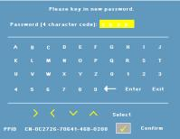
Enable the Password function will pop-up a character screen, key in a 4b digit number from the screen and press the Enter button.
